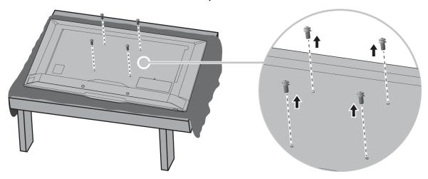
**4** Attach the wall-mount bracket using the screws you removed or the screws that came with the wall-mount bracket. See the instructions that came with the wall-mount bracket for information about which screws to use and how to correctly hang your TV.
